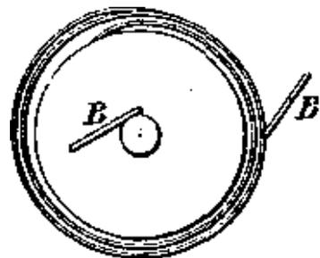
The cores of the magnet are supposed to be hollow, the shaft C of the disc passing through them. If the unmarked pole be below, and the disc be rotated screw fashion, the current will be, as before, from the centre to the periphery, and may be taken off by suitable sliding contacts, B B', on the shaft and periphery respectively. In this arrangement the current flowing through the disc and external circuit will have no appreciable effect on the field magnet.
